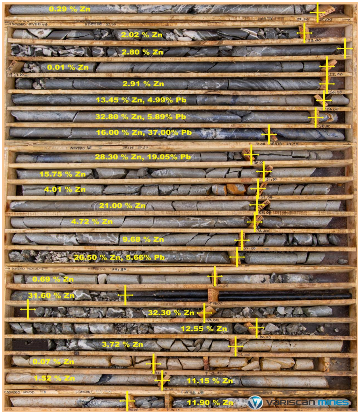
Figure 2. Diamond Drill Core from NOVDD046 illustrating massive sphalerite in dolostone
